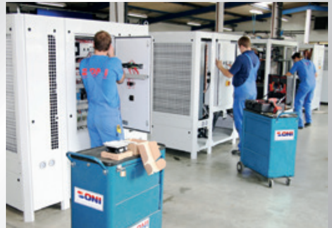
Luftgekühlte Kompakt-Kältemaschine in der Endmontage Air-cooled compact chiller in its final assembly
